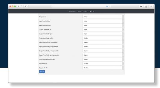
parameters and has features that simplify installation, use, and enhance system performance. A notable feature within the interface is the Automatic Gain Control (AGC). The IBUC continuously monitors input and output levels. When AGC is enabled, the gain of the system is maintained at a constant level by an internal algorithm.
