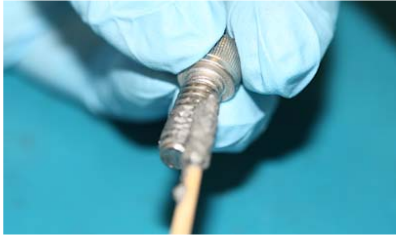
Figure 3.6 Applying the Anti-Seize Lubricant
