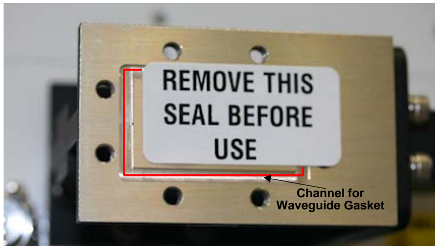
Figure 3.7 Waveguide Label and Channel for Gasket
