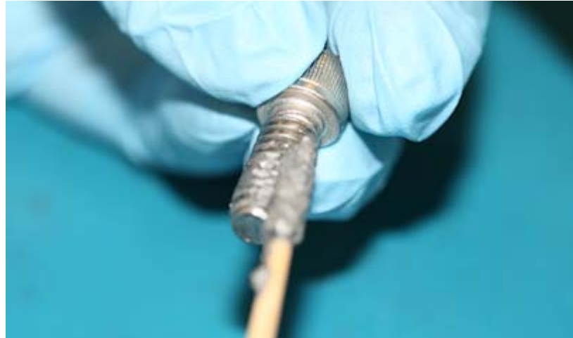
Figure 3.4 Applying the Anti-Seize Lubricant
