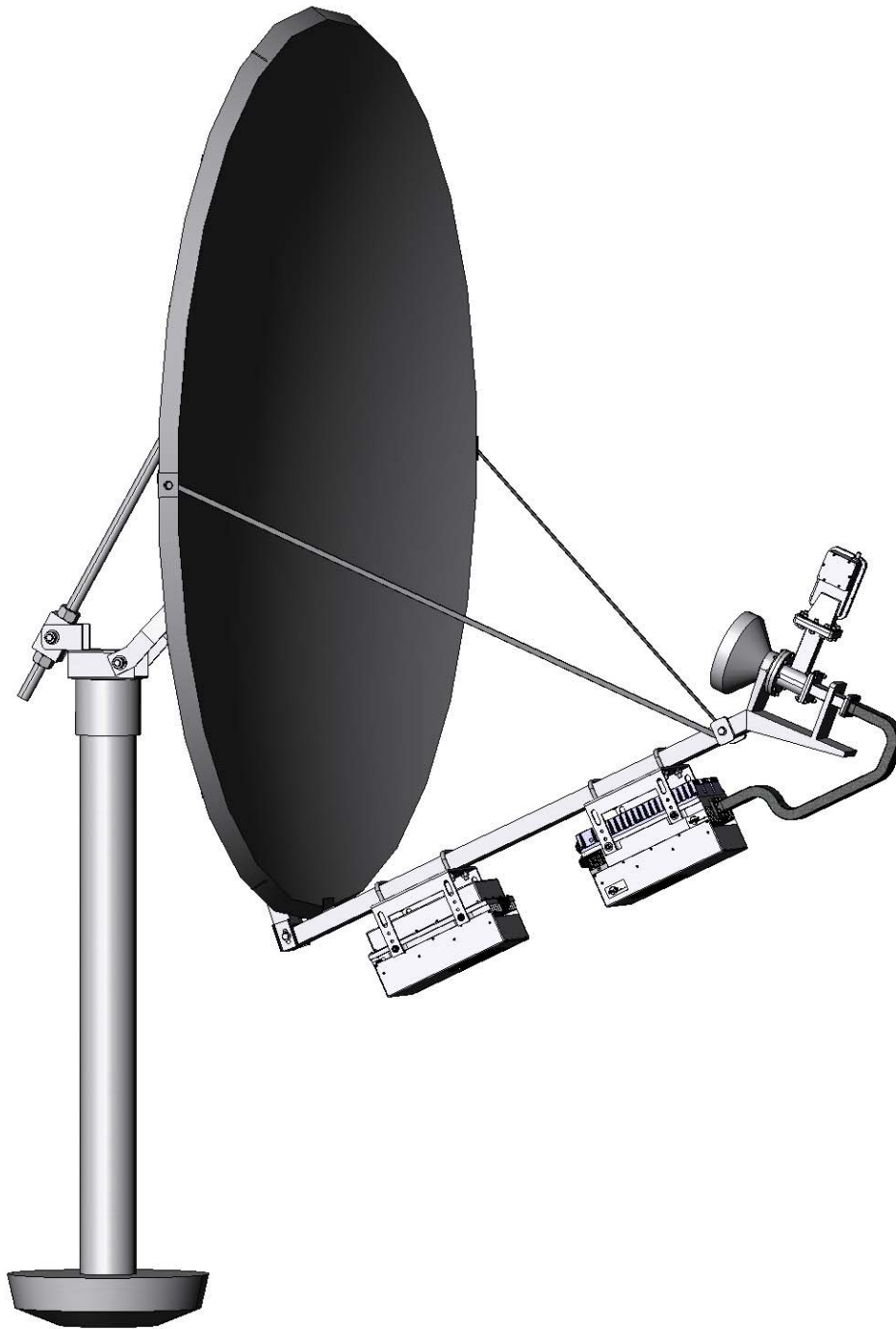
Figure 3.4 Mounting on Boom Arm
