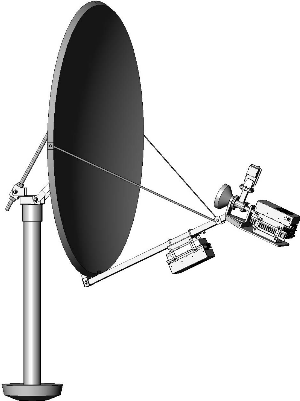
Figure 3.3 Mounting on Focal Point
