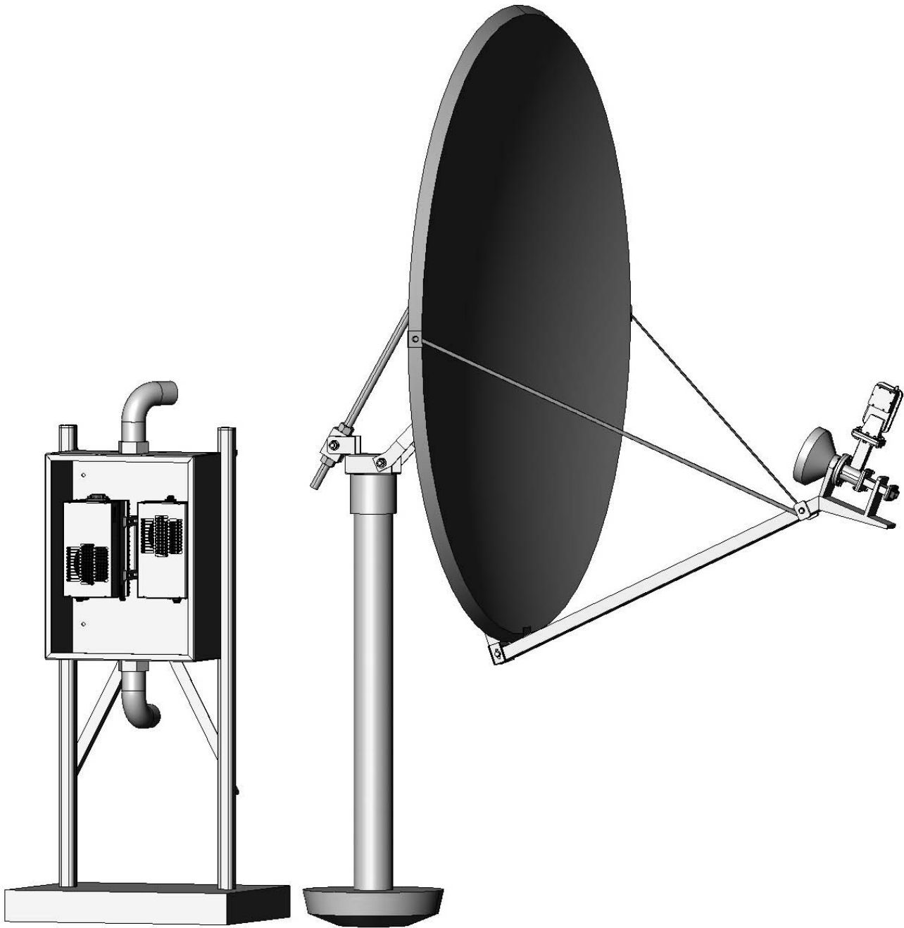
Figure 3.5 Mounting on Antenna Back Structure
