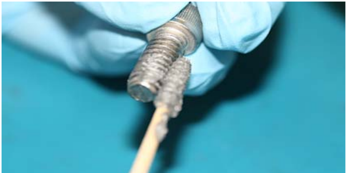
Figure 3.13 Applying the Anti-Seize Lubricant
