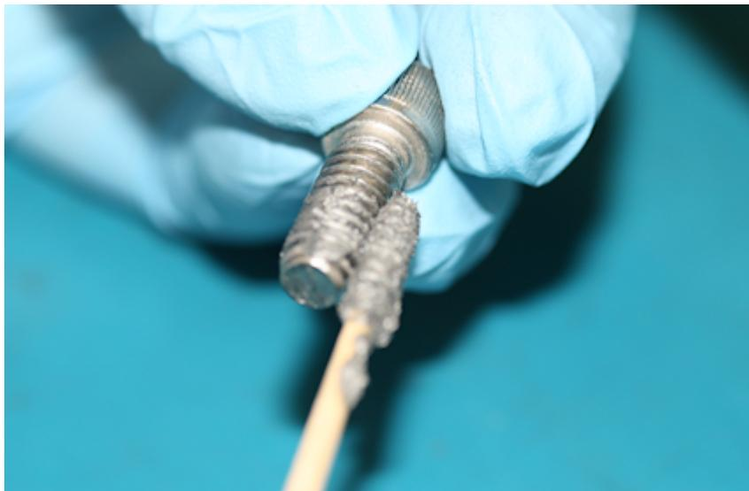
**Figure 3.7** Applying the Anti-Seize Lubricant
