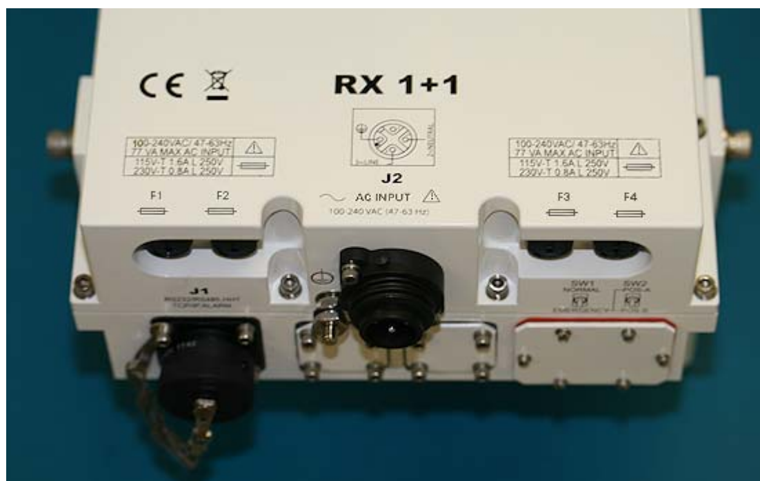
Figure 3.10 Information on Top Cover of an AC-powered Rx 1+1 System
