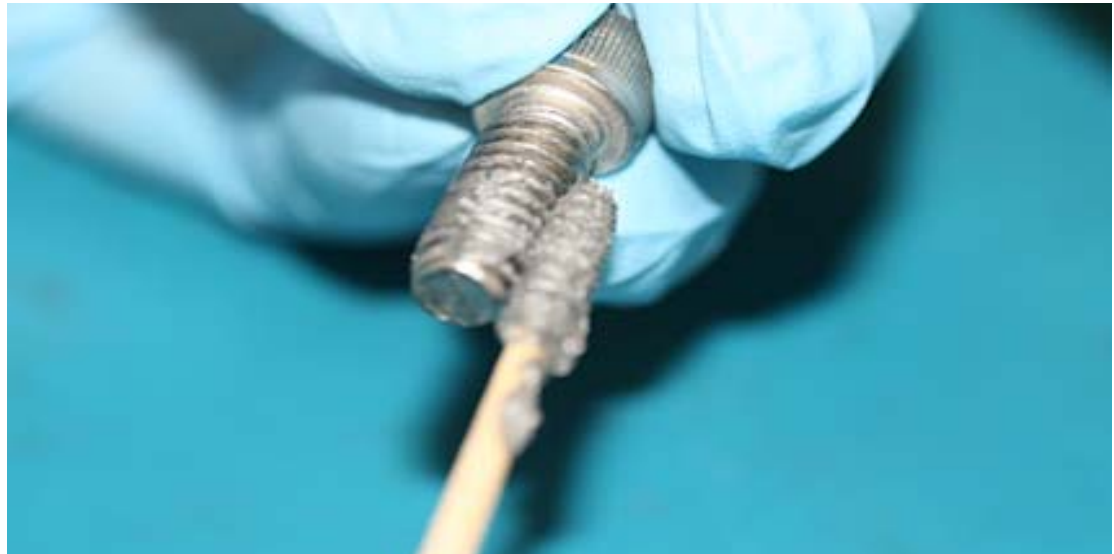
Figure 3.3 Applying the Anti-Seize Lubricant
